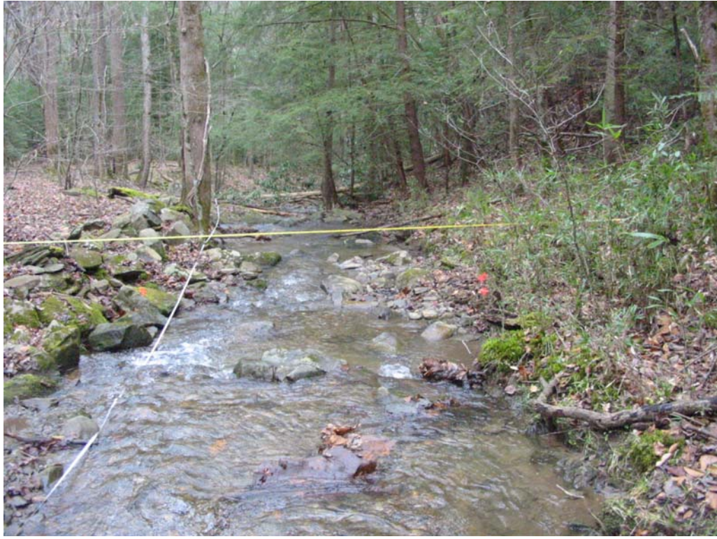
Figure 10. Surveying a monumented cross section.
